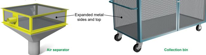
FOX TrimAway's air separator allows conveying air to exhaust to atmosphere while edge trim or other waste "gravity feeds" through the bottom of the unit. It is constructed of expanded metal and is approximately 39" W x 39" x L x 39" H with a 10" diameter opening at the bottom.
